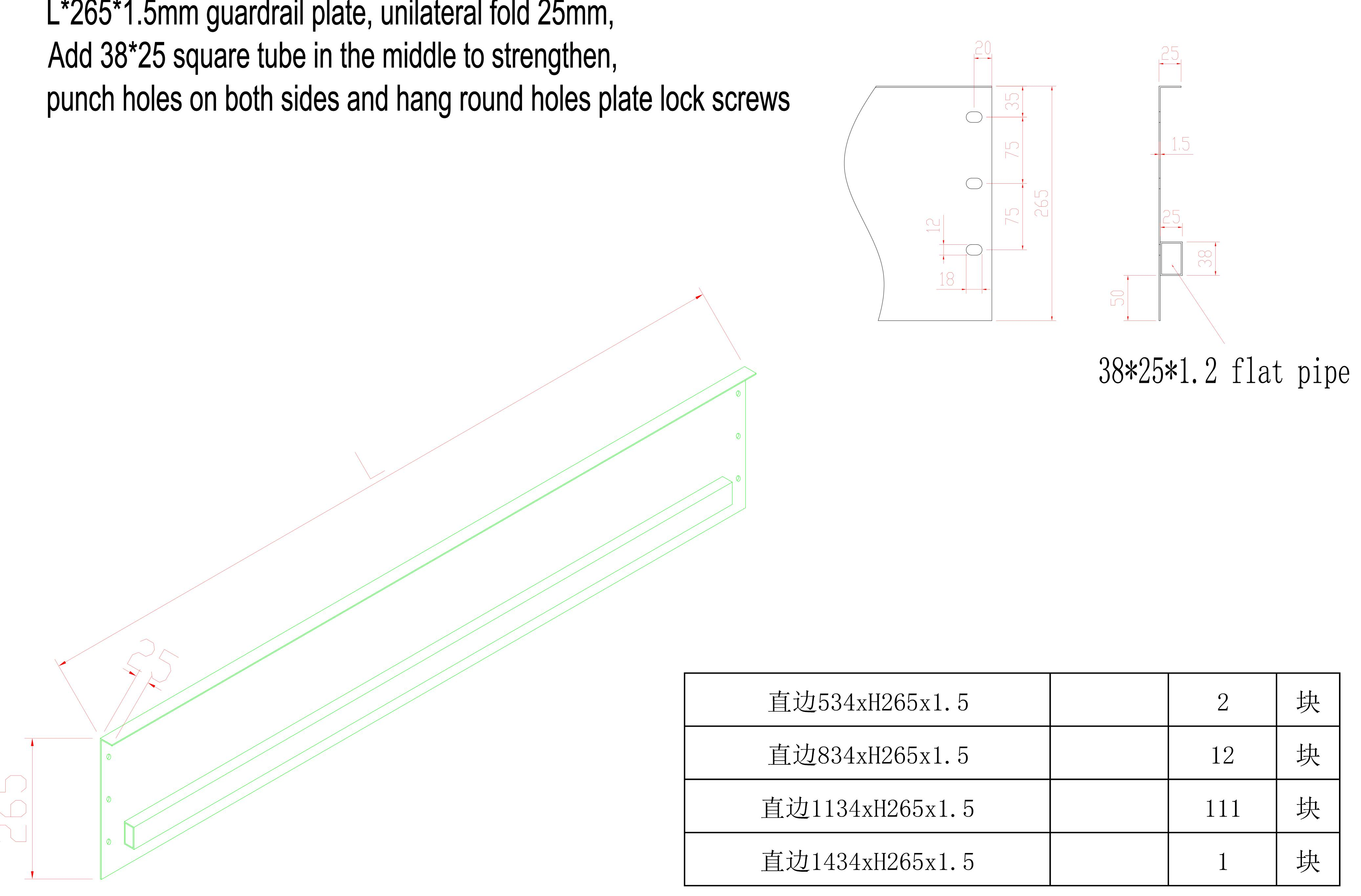
Guardrail baffle (use with guardrail upright)
